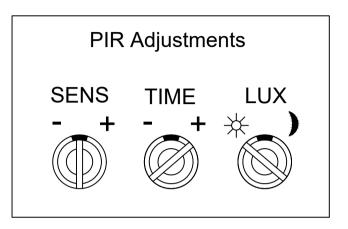
Please Note: After adjusting the PIR please ensure the locking tab that allows you to adjust the angle of the PIR is tightened correctly to ensure the fitting is rated to IP65 failure to do this could result in water ingress and premature failure of the luminaire.
