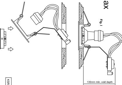
KSRDL101 ØRIm Size 80mm ØCut out (山) 72mm Void Depth Req'd 135mm Max Wattage / Lamp Type GU10 - 50W
