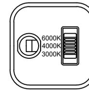
Select Colour Temperature prior to switching on mains supply
